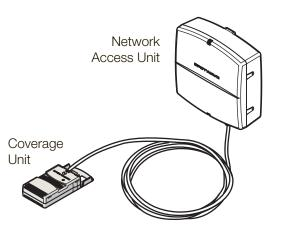
Connect the power cable to the Coverage Unit and then plug the adapter into a power outlet.
