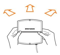
Permanently mount the Network Access Unit on the wall that resulted in the strongest signal level in the coverage area. For mounting options, refer to the User Manual.
