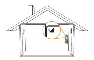
The Network Access Unit direction is a factor in the quality of coverage. You may have to try positioning the unit on different walls to achieve optimal coverage. Try to avoid pointing the Network Access Unit toward the Coverage Unit.
